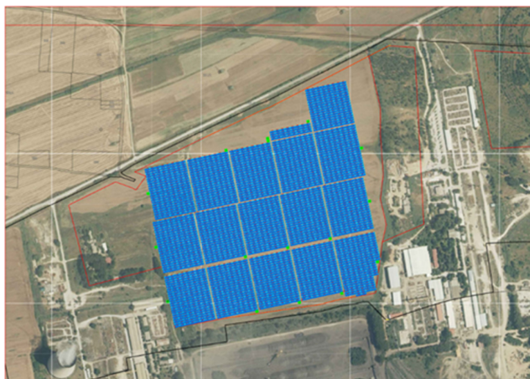
Figure 4.23. Layout of the panels on the site and location of TS of the PhPP Bitola
