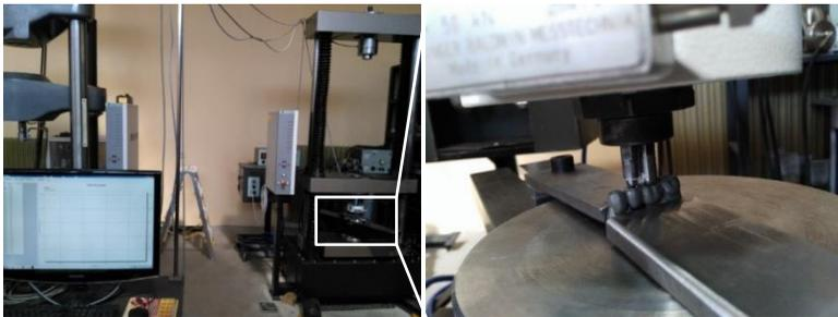
*Fig. 2-15 Bending test of four-part dental bridges.*
