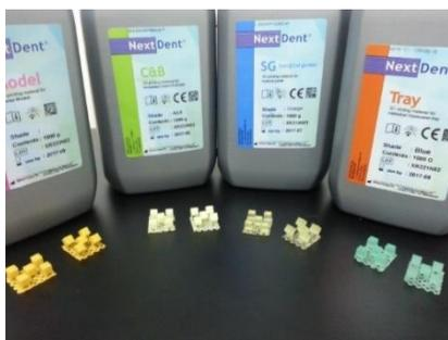
*Fig. 2-1 Cubic samples of different polymers, 3D printed by DLP stereolithography.*
